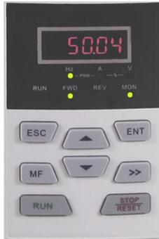
Fig. 4-7 Direct frequency modification status
