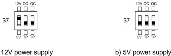
Fig. 3-27 S7 operation when using encoder of differential output type
