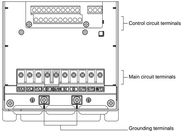
Fig. 3-11 Terminal configuration
