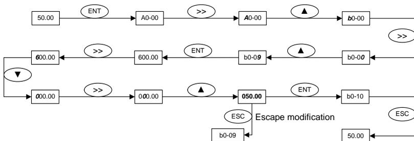
Fig. 4-12 Flow chart of upper limit frequency modification
