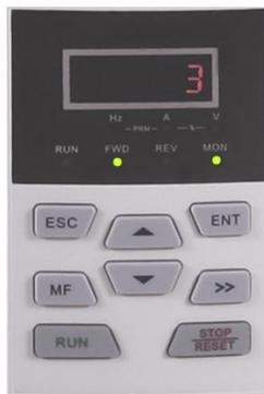
Fig. 4-10 Second-tier display of parameter ("3" is the value of b0-00)
