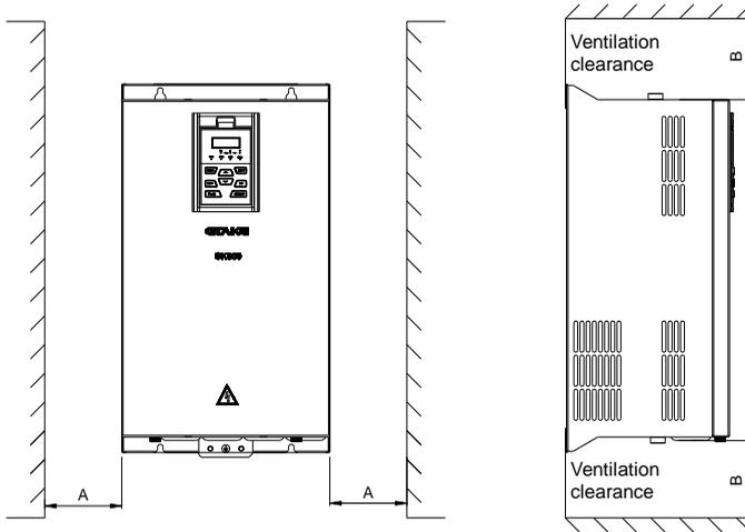
Fig. 3-2 Minimum mounting clearances of GK600-4T18.5G/22L and above
