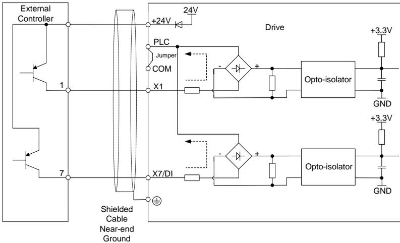
Fig. 3-19 Internal power supply open collector PNP connection
