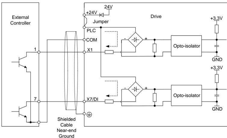
Fig. 3-17 Internal power supply open collector NPN connection
