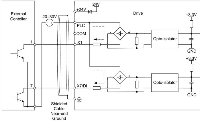
Fig. 3-18 External power supply open collector NPN connection
