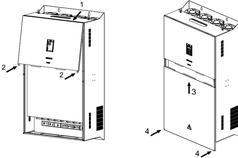
Fig. 3-9 Mount the upper and lower covers
