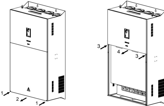
Fig. 3-8 Open the upper and lower covers
