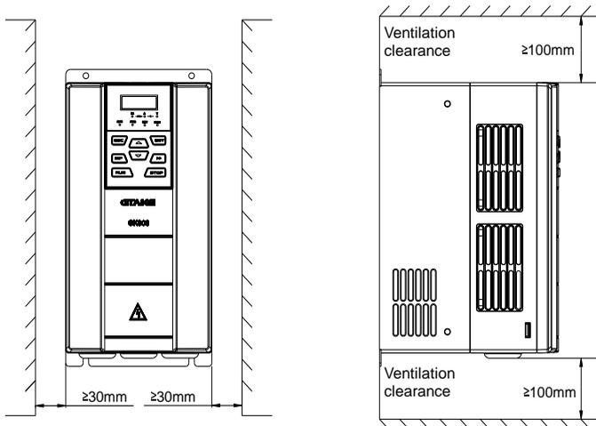
Fig. 3-1 Minimum mounting clearances of GK800-4T15B and below
