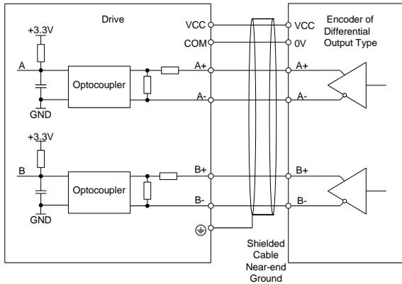
Fig. 3-28 Wiring of encoder of differential output type
