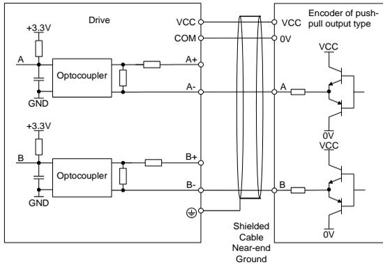
Fig. 3-26 Wiring of encoder of push-pull output type
