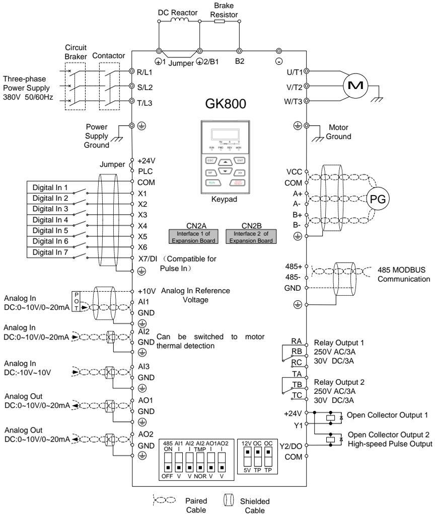
Fig. 3-13 Wiring diagram
