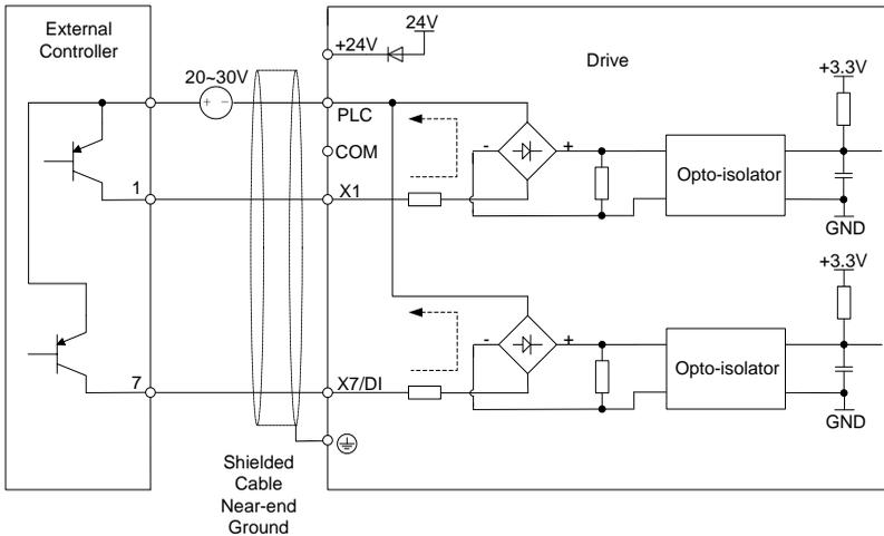
Fig. 3-20 External power supply open collector PNP connection
